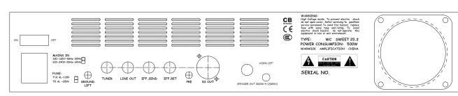
**GROUNDLIFT** switch disconnects the protective ground line from signal ground. A humming loop may occour when
